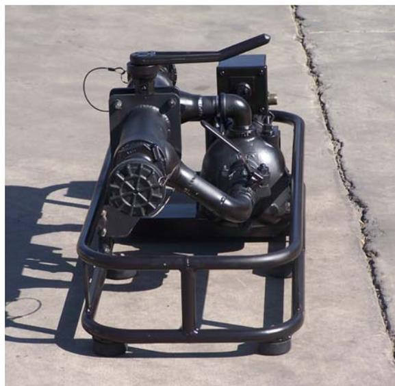
**This unit is electrically-powered (24-28 VDC-from aircraft or HUMVEE) and is configured to allow free flow of fuel through the upper manifold and defuel hoses or pump units after fueling is complete. This is a commercial, off-the-shelf solution to defueling problems, especially in forward areas and uneven terrain.**
